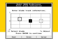
The track information screen, used in rotary wing applications, allows you to enter the blade track information manually, as shown in the example, from visual acquisition using a strobe, or it can be entered for you automatically by the optional Model 540-2 Optical Tracker System. This quick, "paperless" method of recording frees the user from data input. The track information is recorded and can be printed or recalled for later pitch link or tab adjustments.
